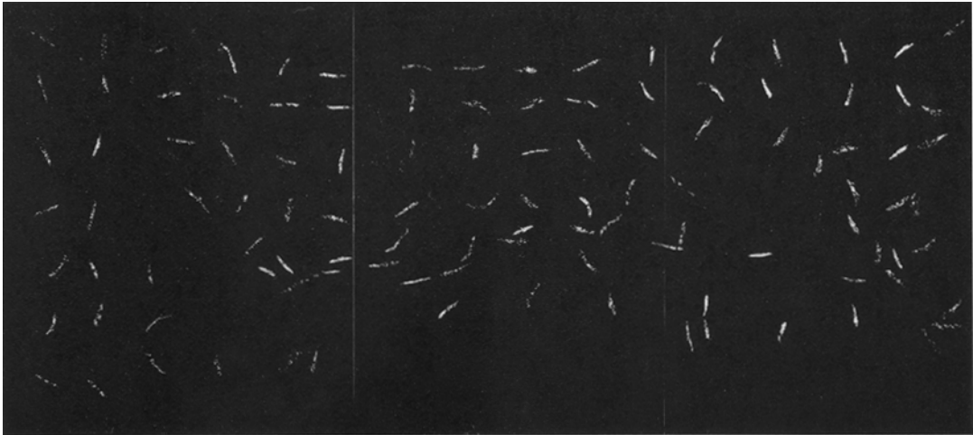
Figure 1 Section of an aligned glass fibre reinforced cement composite taken perpendicular to fibre direction ( \times 5 ).
